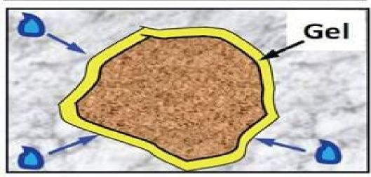
The reaction produces an alkali-silica gel, which absorbs water from the surrounding paste...
