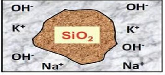
Reaction between the alkali hydroxides (Na, K, & OH) from the cement and unstable silica, SiO<sub>2</sub> in some types of aggregate.
