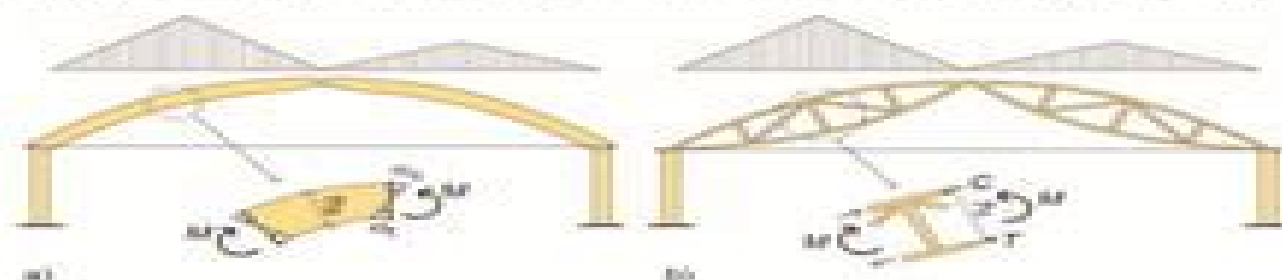
Fig. 21: Arch structures subjected to triangular load distribution. (a) Common arch structure; (b) Arch structure consisting of two laminar trusses connected at the ridge. The effect of relatively large local bending moments M (near \alpha ) can significantly be reduced by closing a structure with larger internal lever arm (case b).
