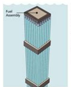
2 After 5-6 years, spent fuel assemblies—typically 14 feet (4.3 meters) long and containing nearly 200 fuel rods for PWRs and 30-100 fuel rods for BWRs—are removed from the reactor and allowed to cool in statage pools for a few years. At this point, the 900-pound (400-kilogram) assemblies contain only about one-fifth the original amount of uranism-235.
