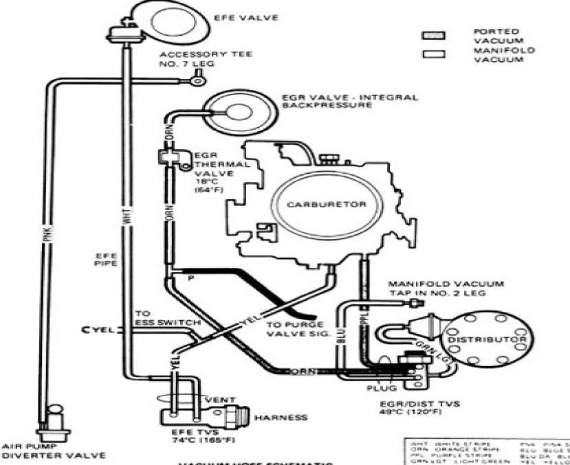
VACUUM HOSE SCHEMATIC (EMISSION SYSTEMS EXCEPT EVAP CANISTER) STRIPE
