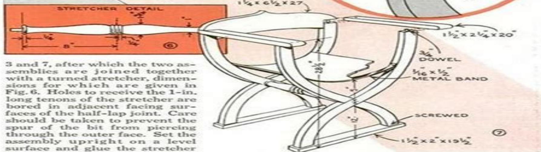
3 and 7, after which the two assemblies are joined together with a turned stretcher, dimensions for which are given in Fig. 6. Holes to receive the 1-in. long tenons of the stretcher are bored in adjacent facing surfaces of the half-lap joint. Care should be taken to prevent the spur of the bit from piercing through the outer face. Set the assembly upright on a level surface and glue the stretcher in place, using a bar clamp as in Fig. 2 to draw the work together tightly.
