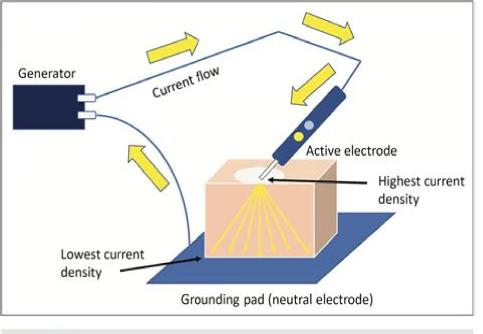
Figure 1: The monopolar electrosurgery circuit..
