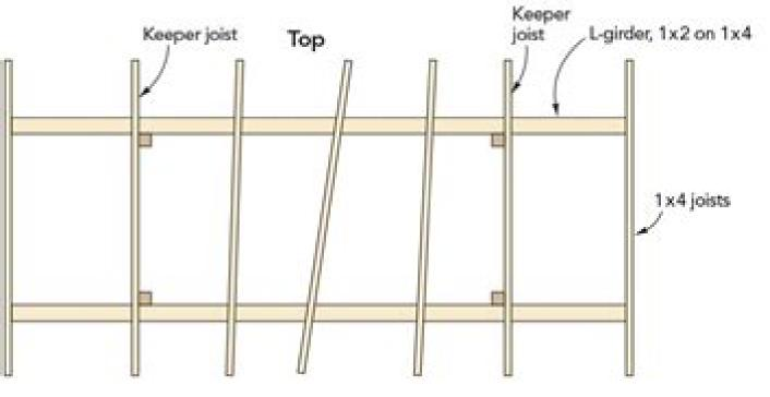
Joists (other than keepers) may be placed at angles
