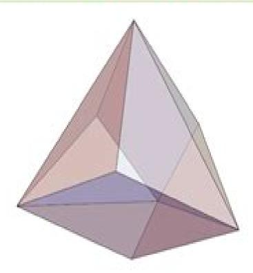
The ten-of-diamonds decahedron is a stereohedron and space-filling polyhedron on 8 vertices, 16 edges, and 10 faces (8 of which are non-equilateral triangles and two of which are rhombi). Because it is polyhedron with 10 faces including two opposite diamond-shaped faces. Goldberg (1982. Fig. 10-II) named it after the "ten of
