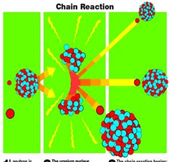
A neutron is about to hit the nucleus of a uranium atom. 2 The uranium nucleus splits (fissions) into several smaller atoms, releasing heat and several more neutrons. The chain reaction begins: those neutrons hit other nuclei, causing them to fission. And so on.
