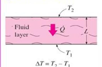
Heat transfer through a fluid layer of thickness L and temperature difference  $\Delta T$ .
