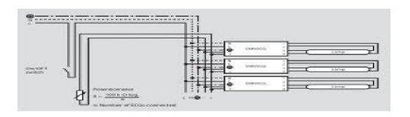
2.2 Systems with up to 50 ECGs with manual control unit DIM . MCU
