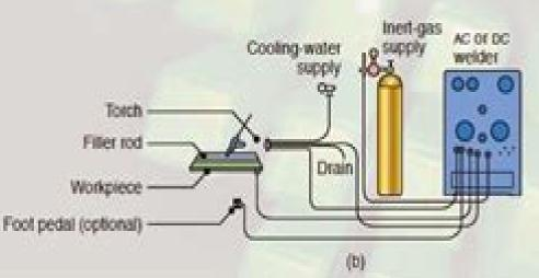
FIGURE 12.11 (a) Gas tungsten arc welding process, formerly known as TIG welding (for tungsten inert gas). (b) Equipment for gas tungsten arc welding operations.
